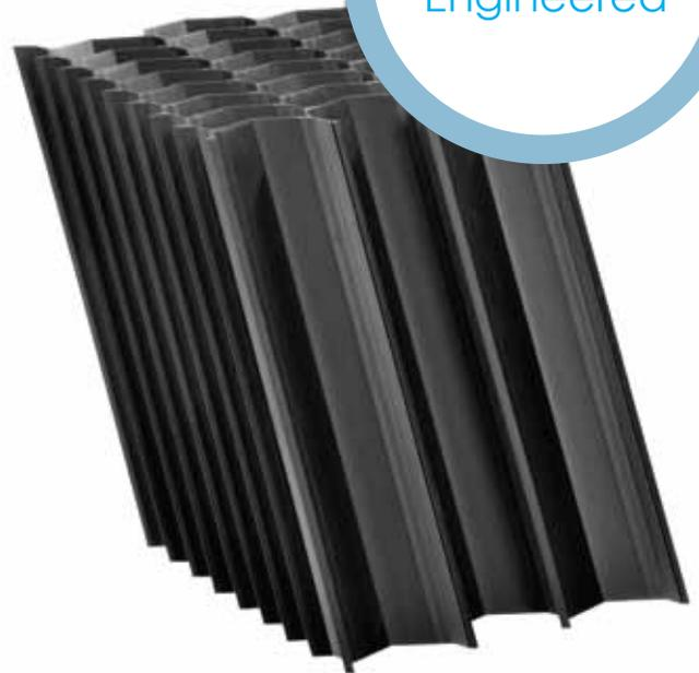
The water entering the plant after screening will still contain high concentrations of sand and silt. Efficient chemical treatment collects the solid material into larger flocculated particles which will settle more readily. Used in conjunction a lamella system, chemical treatment reduces the time needed for particles to hit a solid surface and create a sludge.
